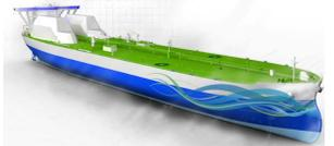
LNG propulsion is one of the key technologies proposed for the 'greening' of shipping.
