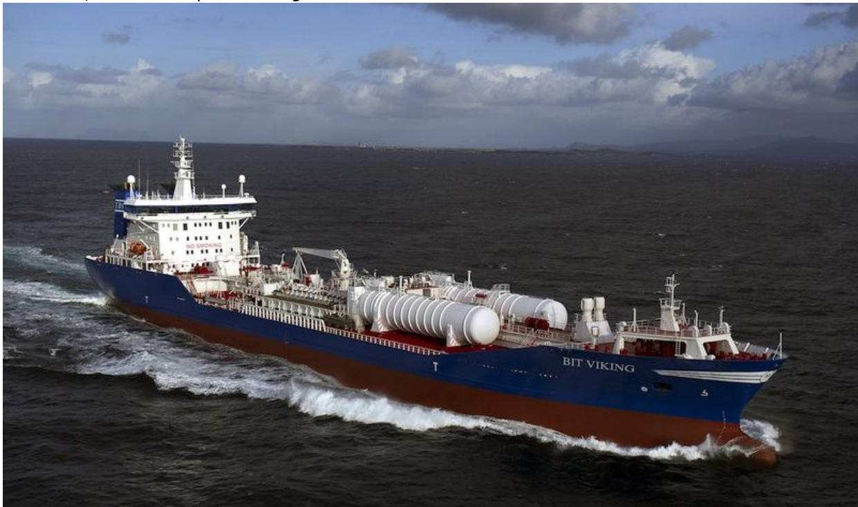
Figure 19 Tanker Bit Viking, converted to run on LNG [Source: Karlsson 2011]
