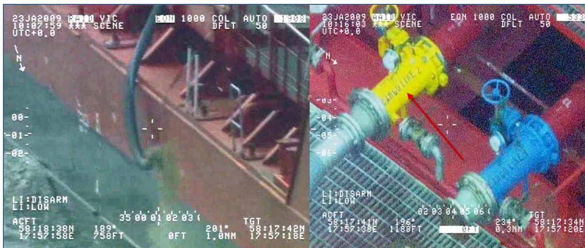
Image 1: Illegal discharge of a MARPOL annex II substance above the waterline
