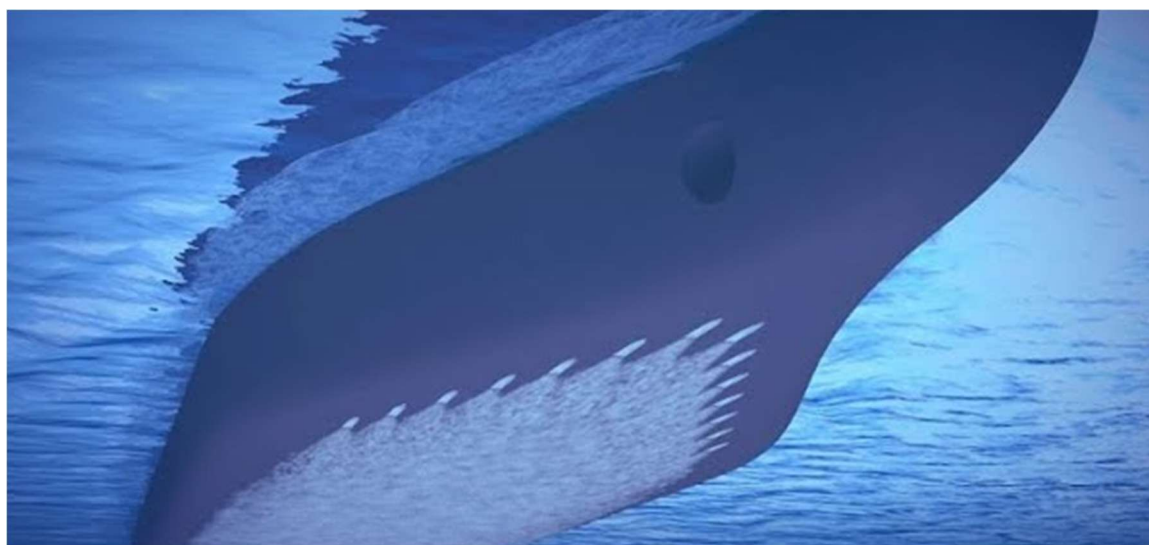
Figure 2-11 Single and V-shaped array of ALS (Source: Silverstream)
