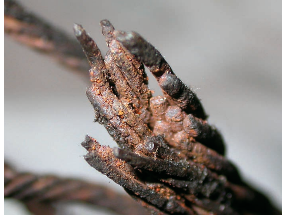
Detail of inner strands of a lifeboat fall wire rope during lab analysis – MV THOMSON MAJESTY.
