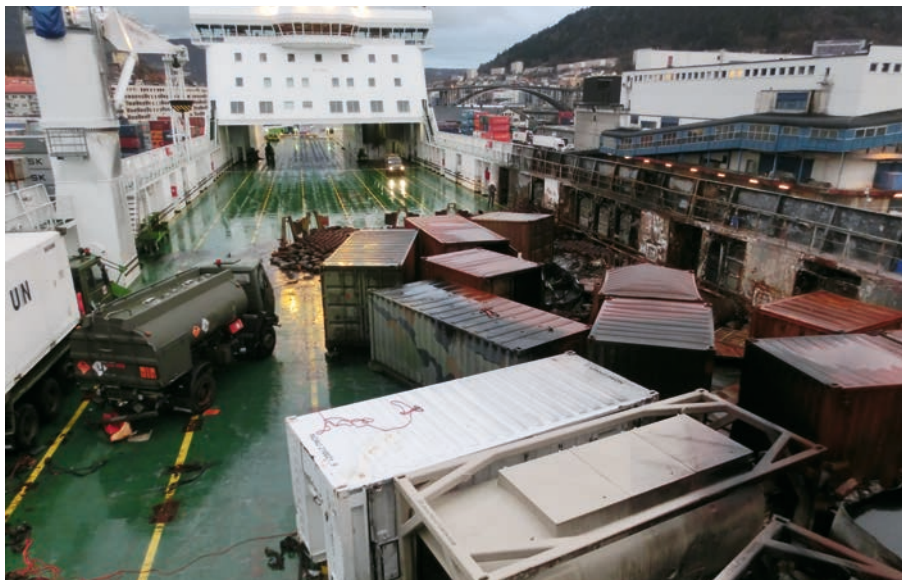
Consequences of a fire at night during rough weather (12 m height waves, 100km/h wind), BRITANNIA SEAWAYS, 16 Nov 2013, less serious occurrence, no injuries, ship damaged, cargo damaged, no pollution.
