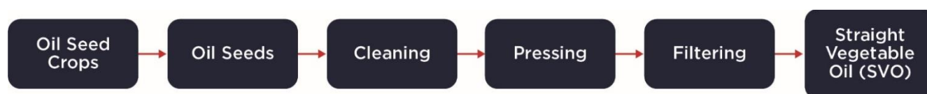
Figure 10. Production steps for Straight Vegetable Oil
