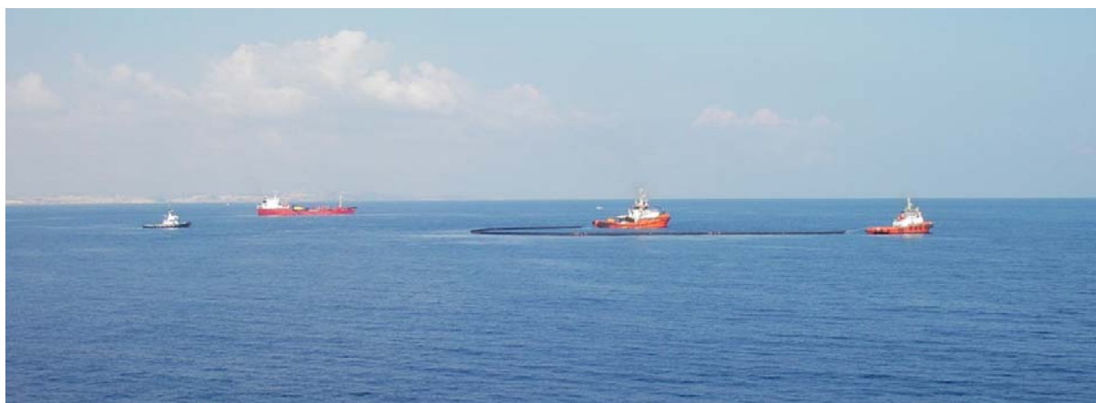
The tugs Spinola and the Felica deploying a boom in J-formation
