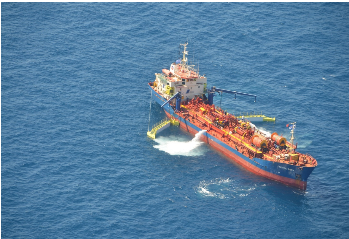
The Aktea OSRV with the sweeping arms deployed during Nireas 2012 exercise
