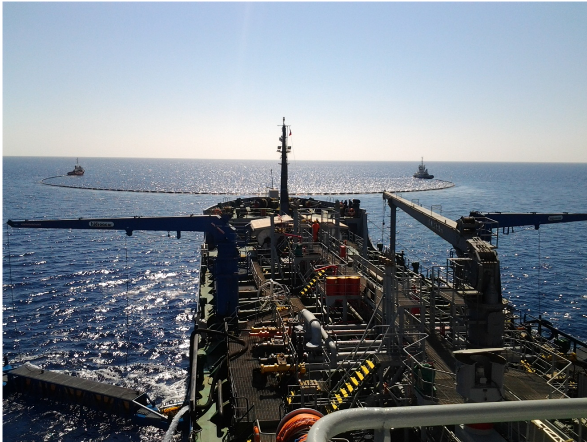
Alexandria following a boom open U-formation with sweeping arms deployed
