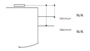
Allowable manifold height above the waterline
