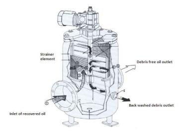
Figure 6: Layout of a self-cleaning strainer (from Fluid Engineering, 2010)
