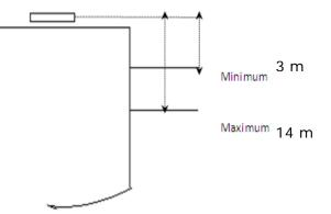
Allowable manifold height above the waterline
