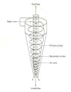
Figure 8: Principle of operation of hydrocyclones (from Unit Operations of Chemical Engineering, 5<sup>th</sup> Edition)
