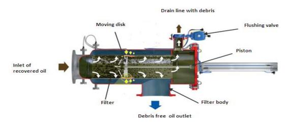
Figure 7: A self-cleaning filter (from Bernoulli AB, 2012)
