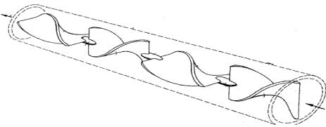
Figure 12: Basic layout of a static mixer (from Stamixco 2007)
