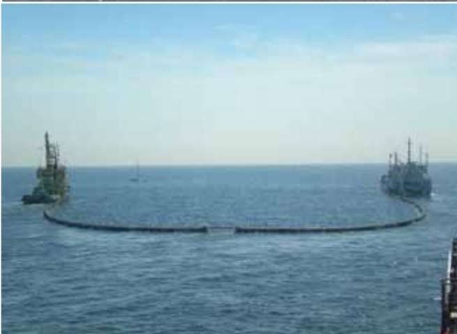
Top: GDC Vlaanderen and Frans Naerebout manoeuvring to form an Open U configuration. Interballast III with sweeping arms manoeuvring to the position behind the Open U for the simulated collection of oil. Bottom left: DC Vlaanderen and Frans Naerebout towing booms in an open U configuration. Bottom right: Inerballast III with sweeping arms in position for simulated oil collection.
