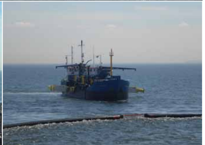
Top: GDC Vlaanderen and Frans Naerebout manoeuvring to form an Open U configuration. Interballast III with sweeping arms manoeuvring to the position behind the Open U for the simulated collection of oil. Bottom left: DC Vlaanderen and Frans Naerebout towing booms in an open U configuration. Bottom right: Inerballast III with sweeping arms in position for simulated oil collection.
