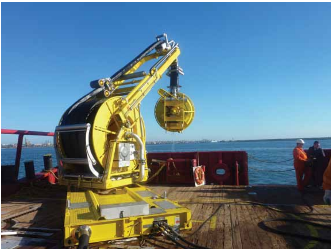
Trans-Rec 150 multi-skimmer on board GSP Orion .
