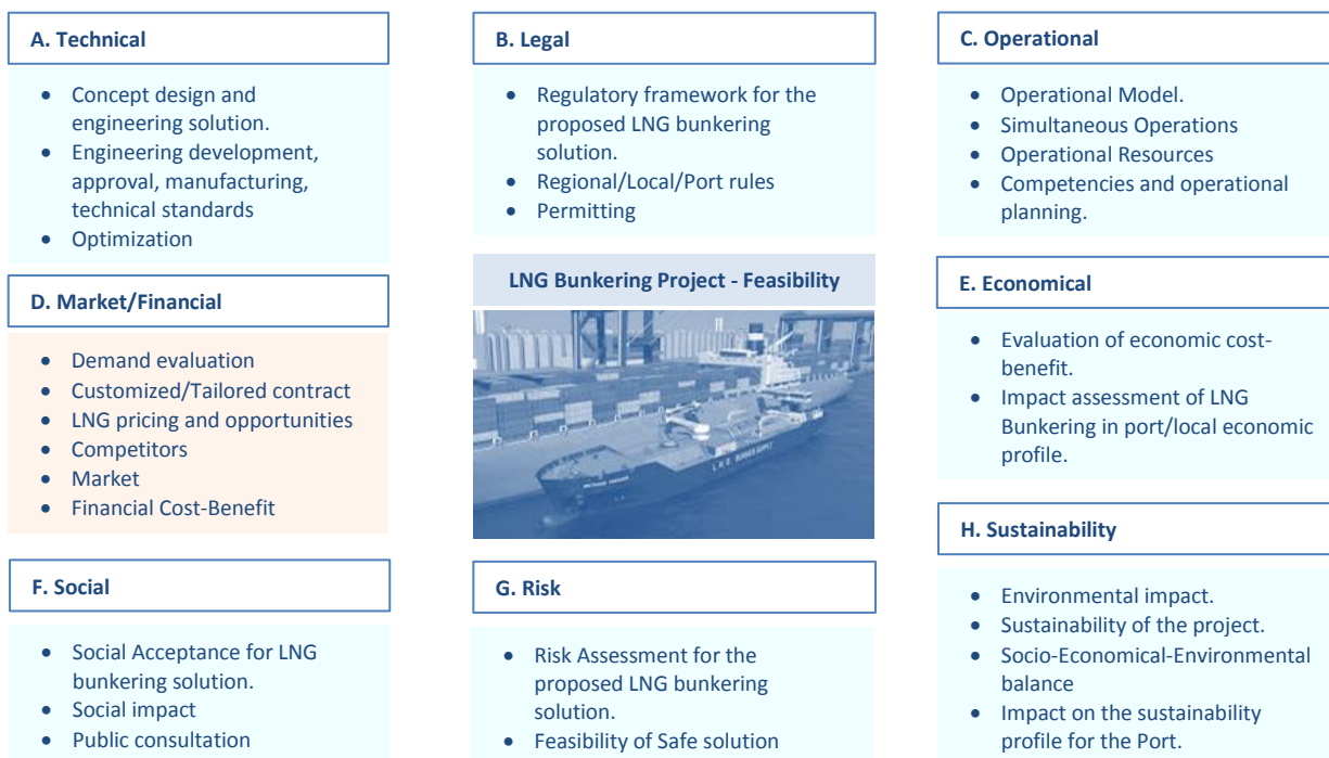
Figure 6.1 – LNG Bunkering project dimensions – Feasibility Analysis In blue all the dimensions that are considered within the scope of this guidance.
