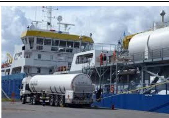
Figure 12.1 – TTS Bunkering. Truck-to-ship LNG delivery of LNG, with truck ashore, alongside of the ship, at berth.
