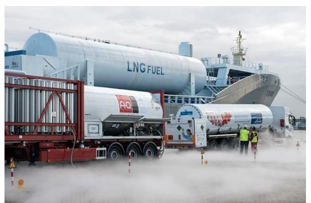
Figure 12.4 – TTS Bunkering. Truck-to-ship LNG delivery of LNG, with truck ashore. It can be noted from this figure how the footprint of the LNG TTS operation may affect the quayside availability for any other operations.
