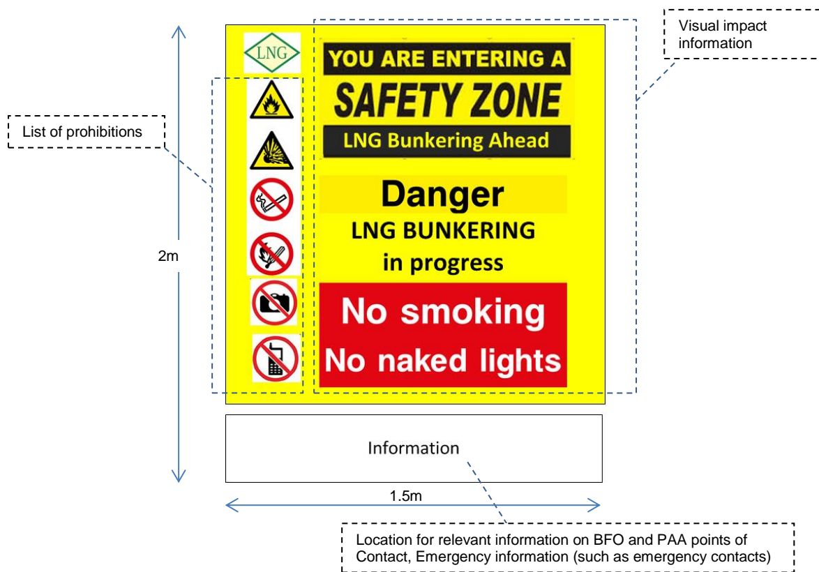
Figure 9.18 – LNG Bunkering Safety Zone notice – Suggested notice at main safety zone entrance points. Main objective is to support the actual control in the implementation of the Safety Zone, through an adequate level of warning/ information.
