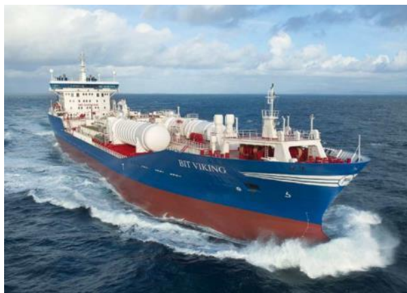
Fig 2.1 – MS BIT Viking – First ship converted to LNG power. [19]. The conversion involved installation of new dual fuel engines and LNG fuel system
