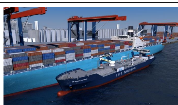
Figure 12.12 – Ship-to-Ship (PTS) Bunkering.
