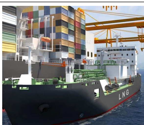
Figure 11.2 – Artist representation of LNG bunker vessel, in STS LNG bunkering onto containership, at berth in container terminal. (source: Shell)
