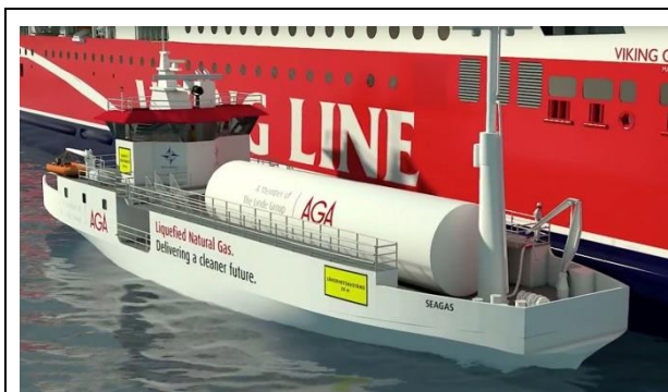
Figure 12.11 – Ship-to-Ship (PTS) Bunkering.
