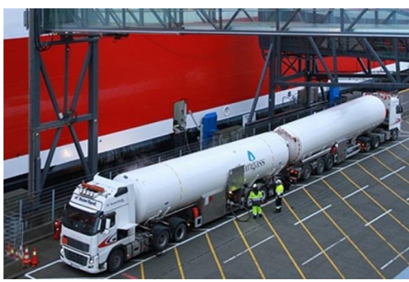
Figure 12.3 – TTS Bunkering. Two truck via comon bunkering manifold.
