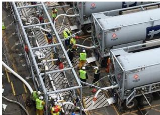
Figure 12.5 and 12.6 – TTS Bunkering by multiple trucks, via common manifold. It can be seen how the complexity of the operation is increased, not only with significant number of connection to common manifold but also with a significant number of personnel. To the technical challenge there is also an organizational one.
