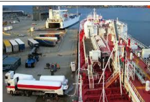
Figure 12.2 – TTS Bunkering. Truck-to-ship LNG delivery of LNG, with truck ashore. Additional truck for inerting.
