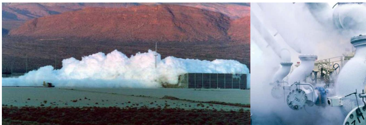
Figures 2.13 and 2.14 – LNG cloud formation and progression (on the left) opposed to the condensation cloud formation around LNG piping due to water vapour condensation in the air surrounding the cryogenic cold piping system.
