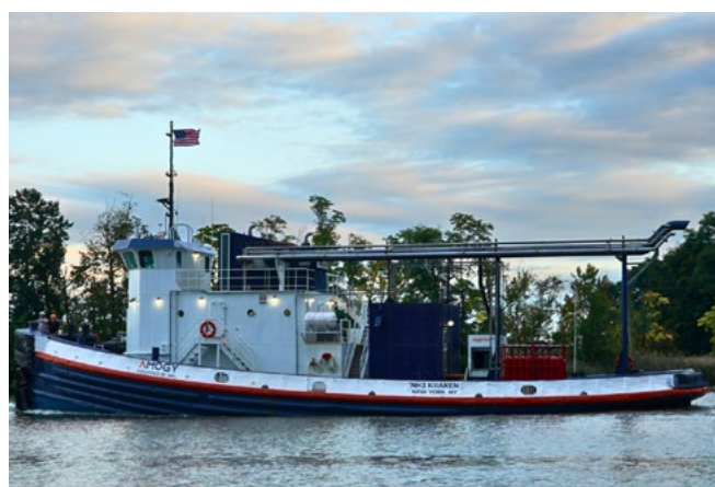
Image 14: The NH3 Kraken, a tugboat originally constructed in 1957 and retrofitted with an ammonia-to-electrical power system.
