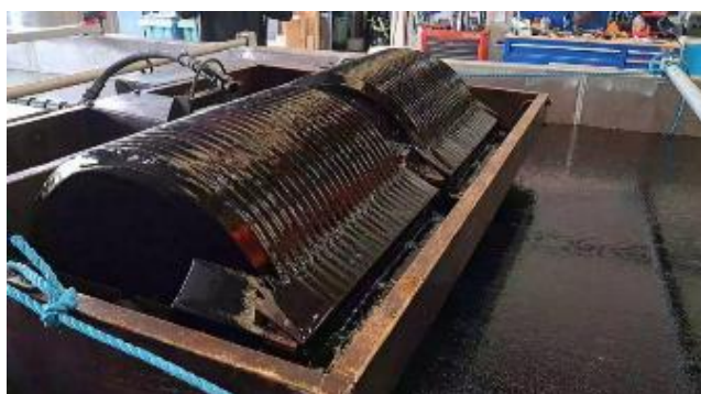
Figure 4. Elastec TDS 118 G skimmer during emulsified B30 recovery (test #4), ©Cedre.
