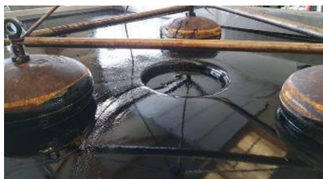
Figure 5. Foilex Mini skimmer during fresh B30 recovery (test #2), ©Cedre.
