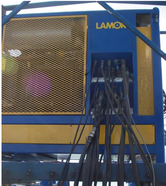
Figure 9 Power pack hydraulic connections
