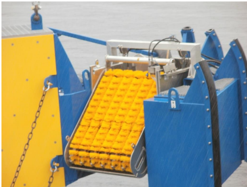
Figure 5 LAMOR Stiff Sweeping Arm LSS 12m – brush skimmer module
