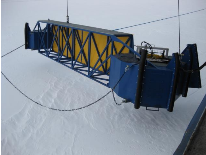
Figure 2 Deployment on ice of Lamor Stiff Sweeping Arms
