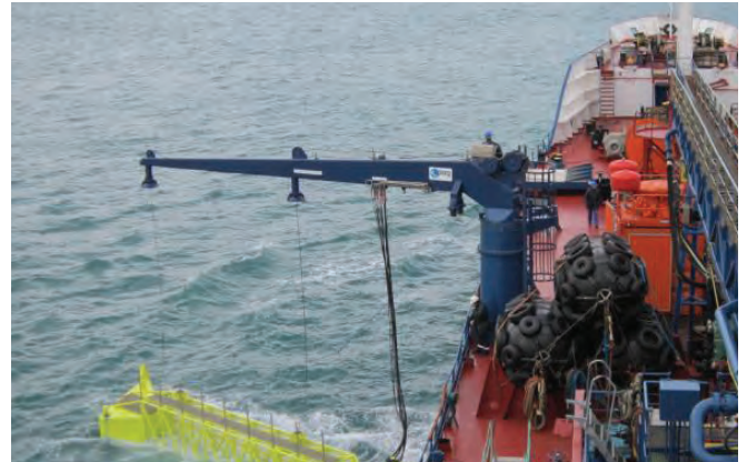
Sara with sweeping arm deployed
