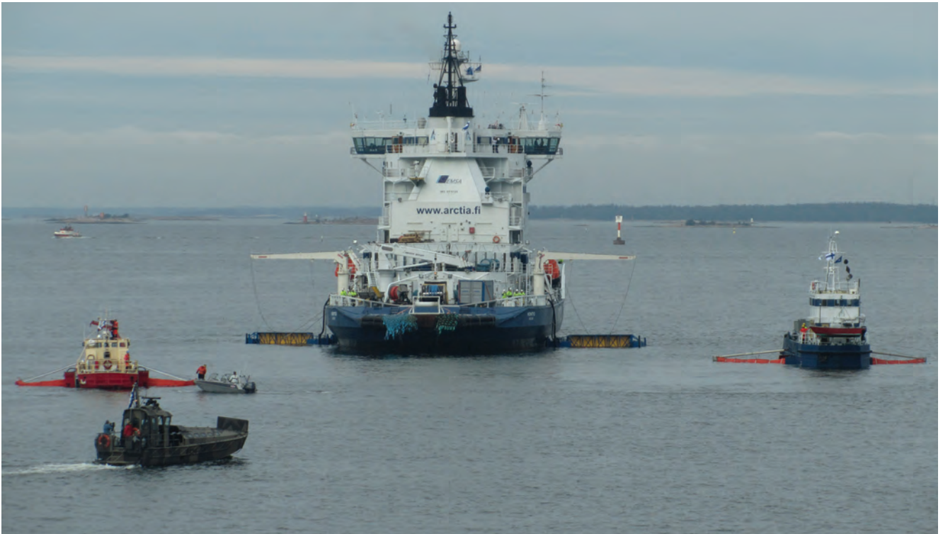
Kontio with sweeping arms deployed during BALEX DELTA 2012
