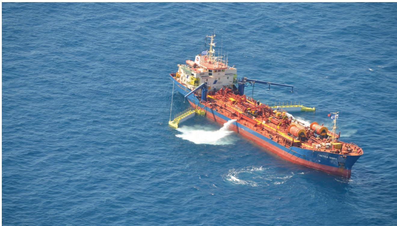
The Aktea OSRV with the sweeping arms deployed during Nireas 2012 exercise
