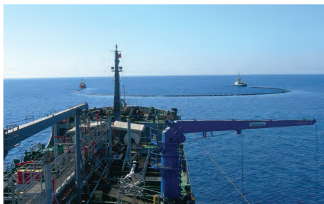
Alexandria following an open "U" formation with sweeping arms deployed
