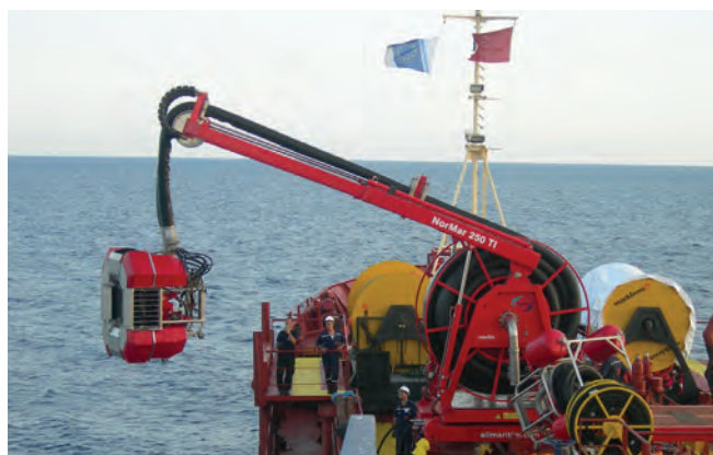
The Aktea OSRV deploying the high-capacity skimmer during the Acceptance Test
