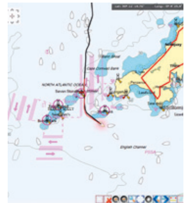
The same information mapped onto a nautical chart showing which vessel is the likely polluter.
