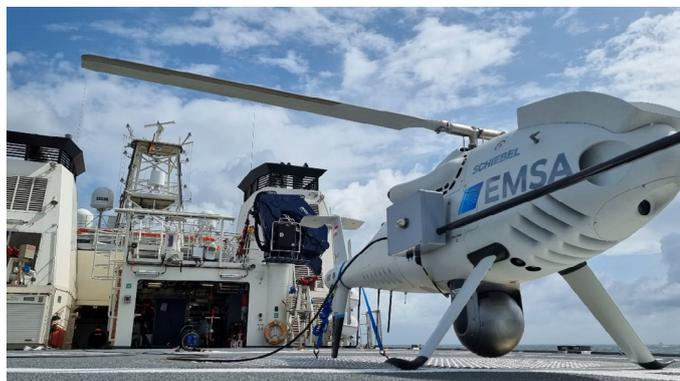
EMSA RPAS located on the helideck of the patrol vessel of the German Federal Police. The air vehicle is equipped with special gas sensors (grey box and pipe on the flank) and optical cameras (turret on the belly). (Photo credits: Schiebel)
