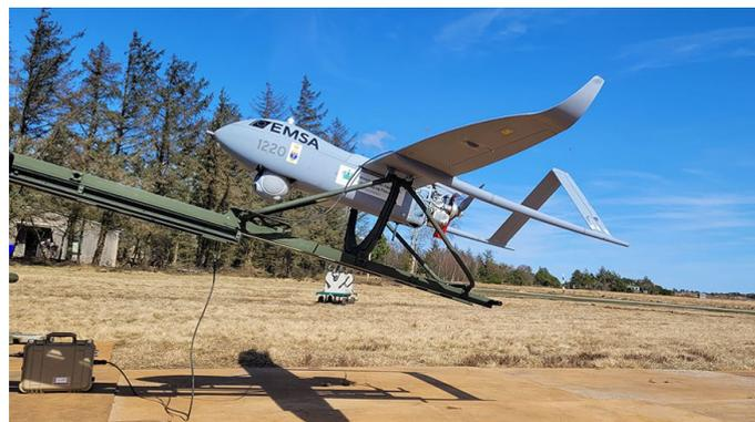
The Aerosonde RPAS uses a catapult for take-off and is recovered with a net. It has an endurance of ten hours and a radio range of 140 km. (Photo credits: EMSA)
